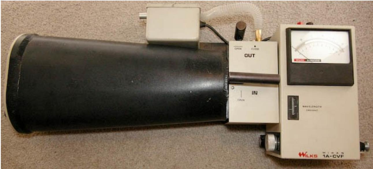
The Miran 1A Infra-red Spectrometer covers wavelengths from 2.5 to 14.5 microns. The cell path length can be varied from 0.75m to 20.5m. This is achieved with gold plated mirrors producing multiple reflections. The Miran 1A is essentially portable provided a source of mains power is available. The output can be recorded with a suitable data logger. The Miran 1A has its own air pump for filling the cell with the sample gas.
