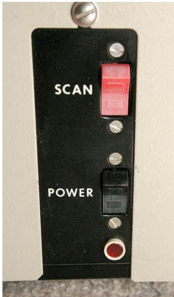
This switch provide a motorised scan of the spectrum and it can be used to produce a spectrum. For best results the sensitivity should be adjusted using a blank spectrum.
