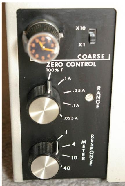
This control adjusts the sensitivity so that the reading is 100% transmission for zero sample. A **x1 or x10 switch** provides a coarse adjustment if necessary.
