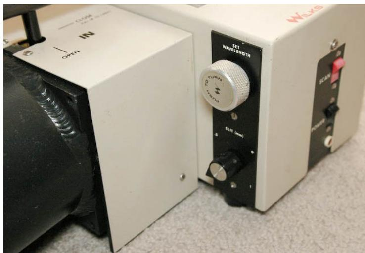
The control for setting wavelength is shown. The control is continuous from 2.5 to 14.5 microns. This range is split into 3 bands seen as you turn the knob. This is because 3 diffraction gratings are used to give good performance over the whole range. The bands cover from 2.5 to 4.5, 4.4-8.0 and 7.9 to 14.5 microns respectively. To convert to  $\text{cm}^{-1}$  simply invert the wavelength in microns and multiply by 10000.
