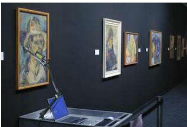
X-ray spectrometry of a Toss Woollaston painting at The Dowse. Some brown spots have formed on the prussian blue area where the measurement is being taken.
